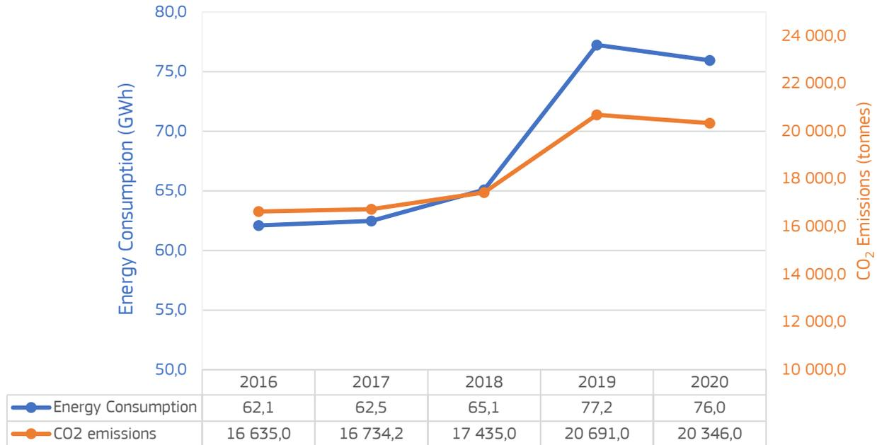
Figure 6 - Temporal evolution of Energy consumption and CO<sub>2</sub> emissions due to maritime transport.
