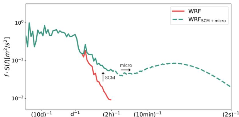
Figure 11. The spectrum of the WRF model and the resulting spectra of the two-step spectral corrections.
