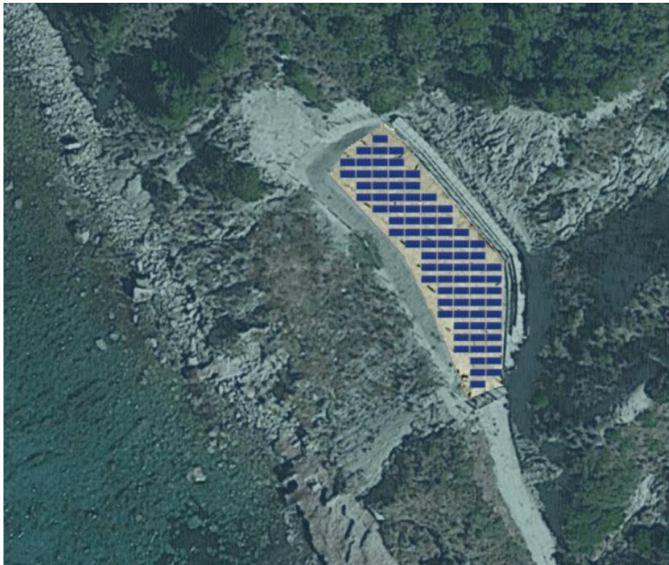
Figure 5 - 44,55 kWp solar modules layout, south facing.
