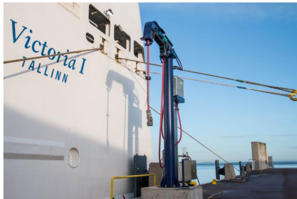
Figure 6: Fixed cable crane (Shore-Link 28 )
