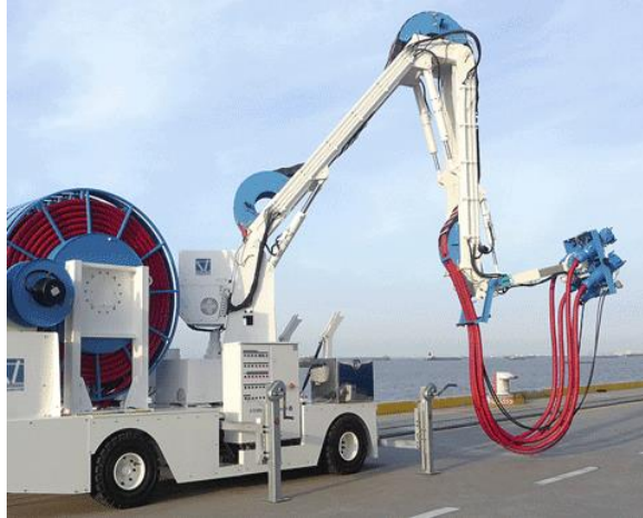
Figure 7: Mobile carrier system for onshore power supply (ShoreCONNECT 29 )
