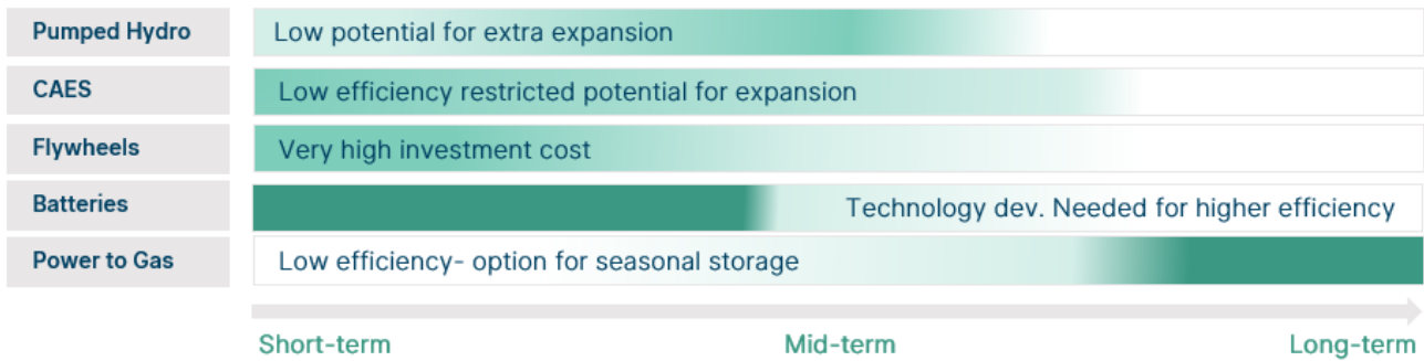
Figure 4: Comparative review of common ESS technologies.
