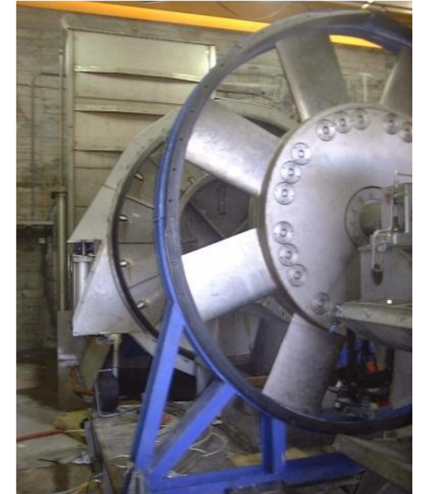
Equipped with a Wells turbine – key component
