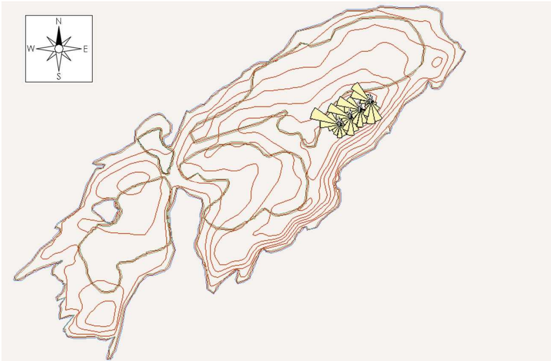
Figure 11a: Wind-roses at the installation positions of 4 wind turbines of 50 kW nominal power each at the southern mountain ridge of the Cape Clear Island.
