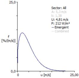
**Figure 13b**: Annual Weibull distribution for wind velocity the installation position of the first wind turbine 3MW.
