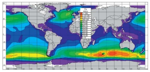
**Figure 20**: Global distribution of annual average wave power density (in kW/m) based on 10-year measurements [12].
