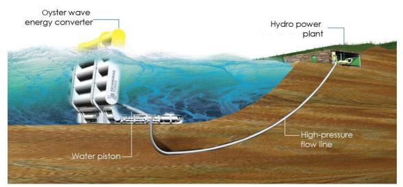
Figure 48: Operation concept and the constructive structure of th an impact wave energy converter [35].
