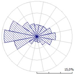
**Figure 13c**: Annual wind rose for the installation position of the second wind turbine 3MW.
