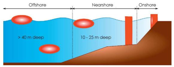
Figure 32: Classification of wave energy converters versus the installation location [14].
