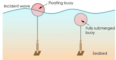
Figure 35: Operation concept and the constructive structure of an point absorber WEC [24].
