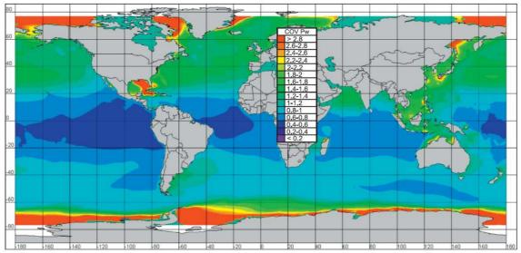
Figure 22: Global fluctuation of the ratio CoV based on 10-year measurements of the wave power density [13].
