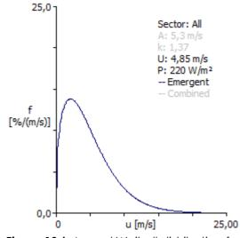
**Figure 13d**: Annual Weibull distribution for wind velocity the installation position of the second wind turbine 3MW.
