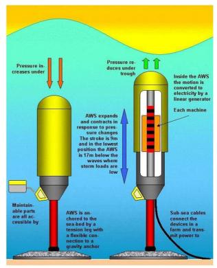
**Figure 37**: Operation concept and the constructive structure of a AWS converter [26].
