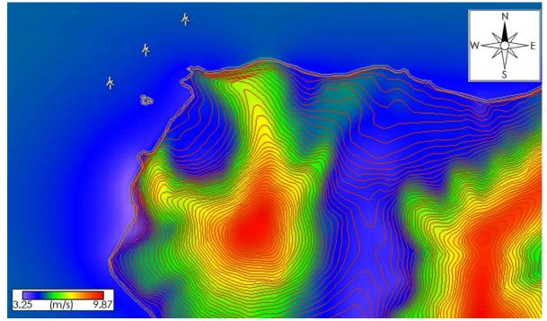
**Figure 11**: Wind potential map and siting of 3 wind turbines of 3 MW nominal power each at the western coast of Salina.
