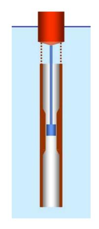
Figure 44: The two-body heaving buoy designed by Sven A. Noren [23].
