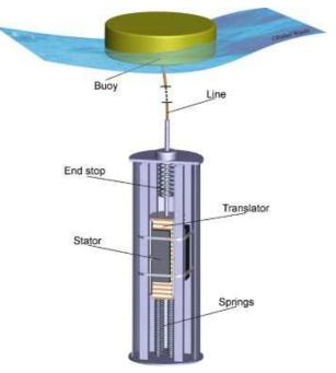
Figure 43: Single-body heaving buoy with linear electrical generator [23].
