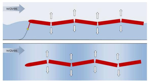
Figure 33: Operation concept and the constructive structure of an attenuator WEC [22].
