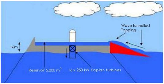
Figure 36: Operation concept and the constructive structure of a terminator WEC [25].
