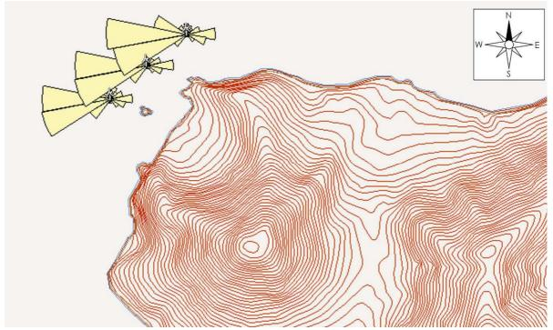
Figure 12: Wind-roses at the installation position of 3 wind turbines of 3 MW nominal power each at the western coast of Salina.
