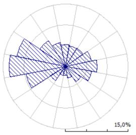
**Figure 13a**: Annual wind rose for the installation position of the first wind turbine 3MW.
