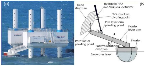
Figure 46: Operation concept and the constructive structure of the WaveStar floating converter [32].
