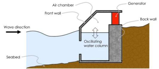
Figure 38: Operation concept and the constructive structure of a OWC converter [27].
