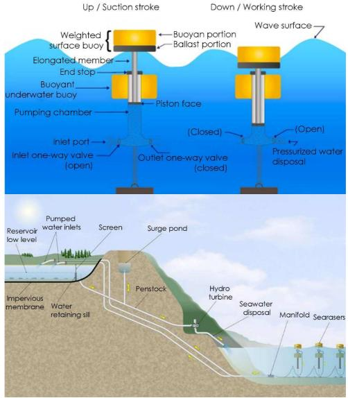
Figure 45: Operation concept and the constructive structure of the Searaser floating converter [30, 31].
