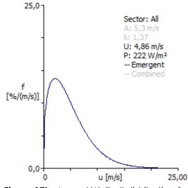
**Figure 17b**: Annual Weibull distribution for wind velocity the installation position of the first wind turbine 5MW.
