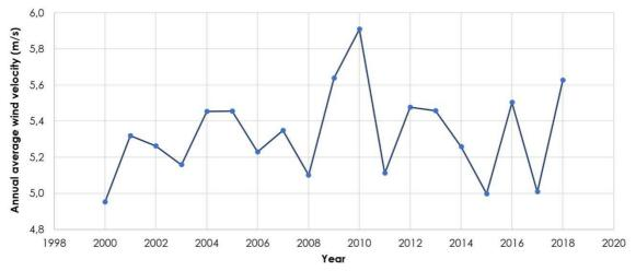
**Figure 4**: Fluctuation versus time of the annual average wind velocity at the wind potential measurement point and at 100 m height above sea level [3].
