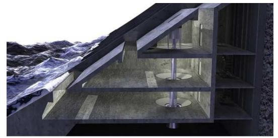
Figure 47: Operation concept and the constructive structure of the SSG wave energy converter [34].
