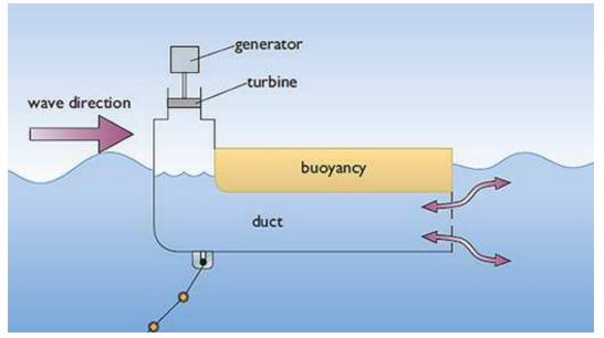
Figure 41: The constructional and operation concept of the Backward Bent Duct Boy [29].
