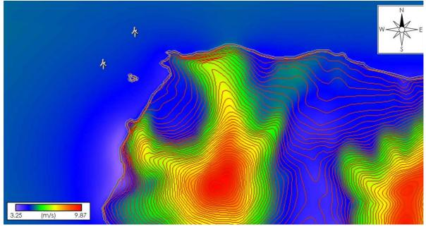
Figure 15: Wind potential map and siting of 2 wind turbines of 5MW nominal power each at the western coast of Salina.
